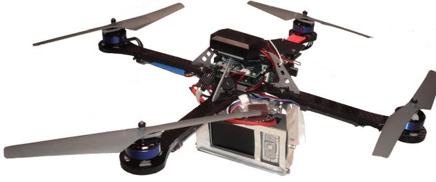
**Fig. 1** The quadcopter Asctec X3D-BL with a Nokia N95 mobile phone.
