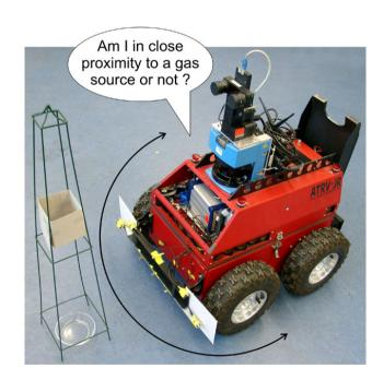
The gas-sensitive mobile robot in front of an object suspected to be a source of gaseous Whiskey.
