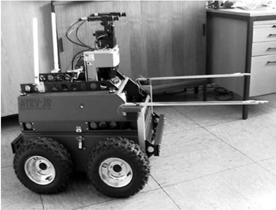
Figure 1: The autonomous mobile robot ARTHUR equipped with an electronic nose. Notice the tube-shaped sensor sticks, which were mounted at the end of the outstanding bars on the front side of the robot.
