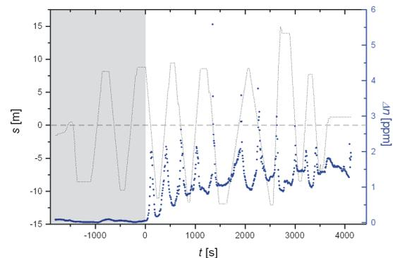
Figure 3: Chemical concentration measurements taken in a corridor in the university building with a robot moving at a constant speed. The gas sensor was placed at the front bumper approximately 30cm in front of the robot's center of mass. A jar with an opening area of 20cm<sup>2</sup> filled with acetone was placed in the center of the corridor ( $s = 0m$ ) at the time  $t = 0s$ . The measured values are indicated by strong dots while the sensors position is drawn in with a thin dotted line.
