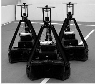
**Figure 4.** Omnidirectional mobile robots used in the formation control experiments.
