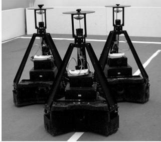
**Figure 4.** Omnidirectional mobile robots used in the formation control experiments.
