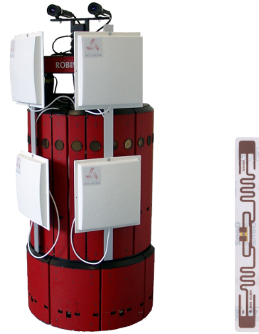
Fig. 1. Left: The RWI B21 service robot employed for our studies, equipped with an UHF RFID reader and two pairs of UHF antennas. Right: The type of tag (“squiggle tag”) that we used for our studies, manufactured by Alien Technology (drawn to a larger scale than the robot on the left). The size of the tag is approximately 10 cm × 1 cm.
