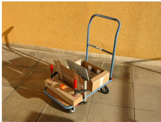
Fig. 3. The experimental cart we used to collect the data. The accelerometer is mounted on the middle of the wooden beam.
