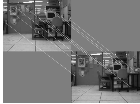
Fig. 11. Matching two images using the iterative SIFT approach with 25 keypoints. There are 11 common keypoints. The distance between the positions of the two images is 18.1 cm.
