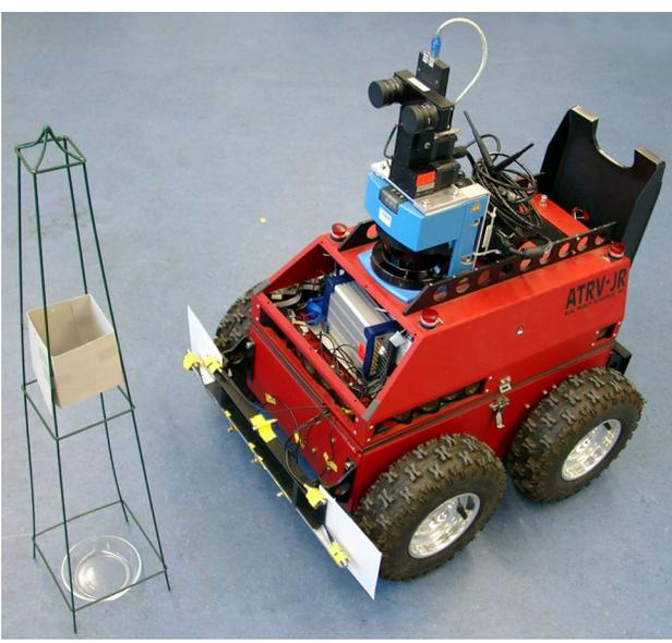
Fig. 1. The gas-sensitive mobile robot Arthur in front of the gas source. This distance was considered as being directly in front of the source.
