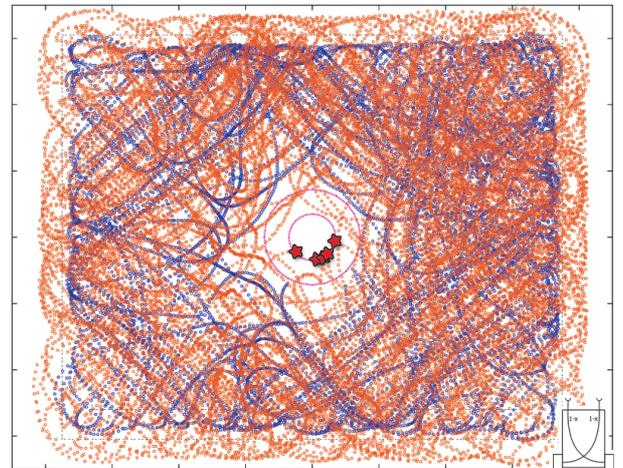
**Figure 7:** Path of a Braitenberg-Vehicle with crossed (1-x)-connections during 3 hours including 5 single trials (collisions are marked by a star). Note that such a plot - i.e., the area which is not covered by the robot - may provide an alternative method to localise the source.
