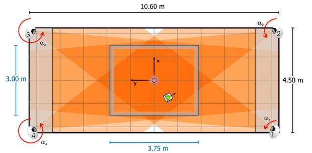
**Figure 3:** Absolute positioning system with 4 cameras. The figure shows a floor plan of the laboratory room and the outline of the region in which the localisation experiments were performed. Also plotted are the fields of view for each camera, shaded according to the number of cameras which can sense a particular region.
