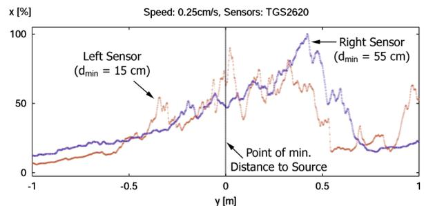
**Figure 1:** Example of gas sensor readings recorded while the robot passed an odour source (ethanol) along a straight line at a speed of 0.25 cm/s. The curve displays relative conductance values of two metal oxide sensors mounted on the left and on the right side of the robot with a separation of 40 cm.
