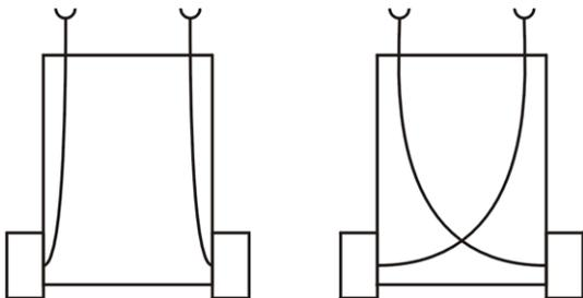
**Figure 4:** Schematic view of Braitenberg vehicles with a direct sensor-motor coupling.
