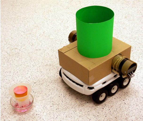
**Figure 2:** The Örebro Mark III mobile nose. Two sets of 3 gas sensors were mounted inside the two suction tubes mounted at the rear of a Koala mobile robot. The picture also shows the odour source and the coloured “hat” used for determining the absolute position of the robot.
