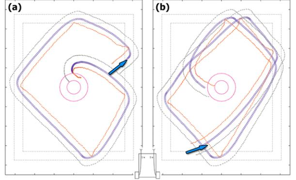
**Figure 5:** Examples of the driven path of a Braitenberg-Vehicle with uncrossed (1-x)-connections (permanent love). The plot shows starting position and initial heading (arrow), the measured location of the robot’s center (circle) and both its front corners (small dots), the virtual repellent walls (broken line) and two circles indicating the location of the source.
