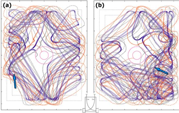
**Figure 6:** Examples of the driven path of a Braitenberg-Vehicle with crossed (1-x)-connections (permanent love). See Fig. 5 for details of illustration.
