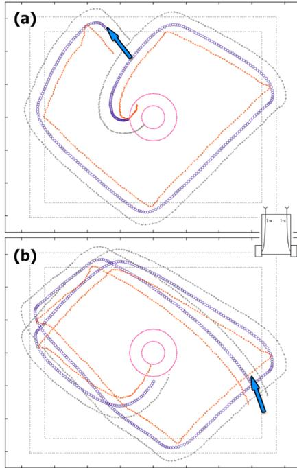
**Fig. 3.** Examples of the driven path of a Braitenberg-Vehicle with uncrossed (1-x)-connections (*permanent love*).
