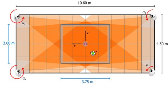
**Fig. 2.** Floor plan of the used laboratory room together with an outline of the area inspected.
