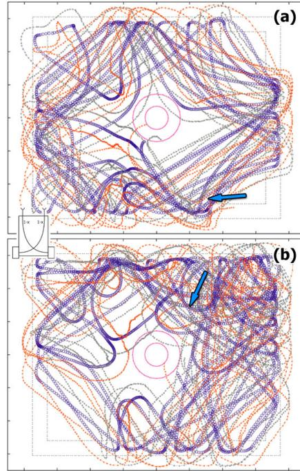
**Fig. 4.** Examples of the driven path of a Braitenberg-Vehicle with crossed (1-x)-connections (*exploring love*).
