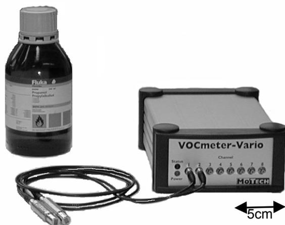
Figure 1: VOCmeter-Vario with two sensor sticks connected via a RG 158 coax cable. It is possible to connect up to eight different sensors. All sensors are driven by the electronics in the main unit. The sensor signals are transmitted to a computer via a serial RS-232 link.
