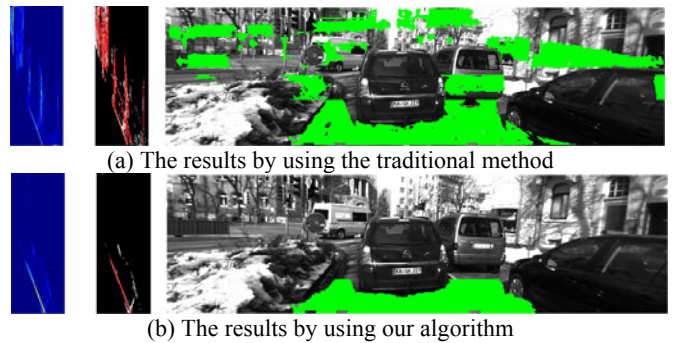
Fig. 10. The comparison between the traditional method [5, 7, 8] and our algorithm (from left to right: the v-disparity image shown by using a pseudo color LUT, the detected ground correlation line, and the detected traversable regions).
