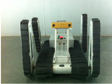
Fig. 1. Our NuBot rescue robot system
